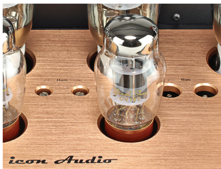
The small valves at front are 6SN7 triodes, known for their deliciously smooth sound. Behind are adjustable hum buckers (left) and adjustable bias potentiometers (right).
