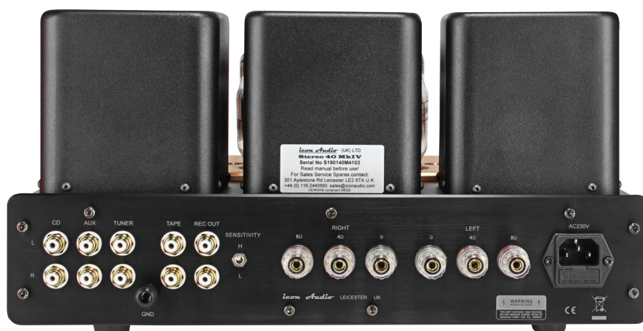
The rear carries heavy duty, gold plated phono socket inputs (left) and equally solid, gold plated loudspeaker terminals for 4 Ohm or 8 Ohm loudspeakers. Above are large in-house designed and built output transformers at left and right, with mains transformer at centre.
