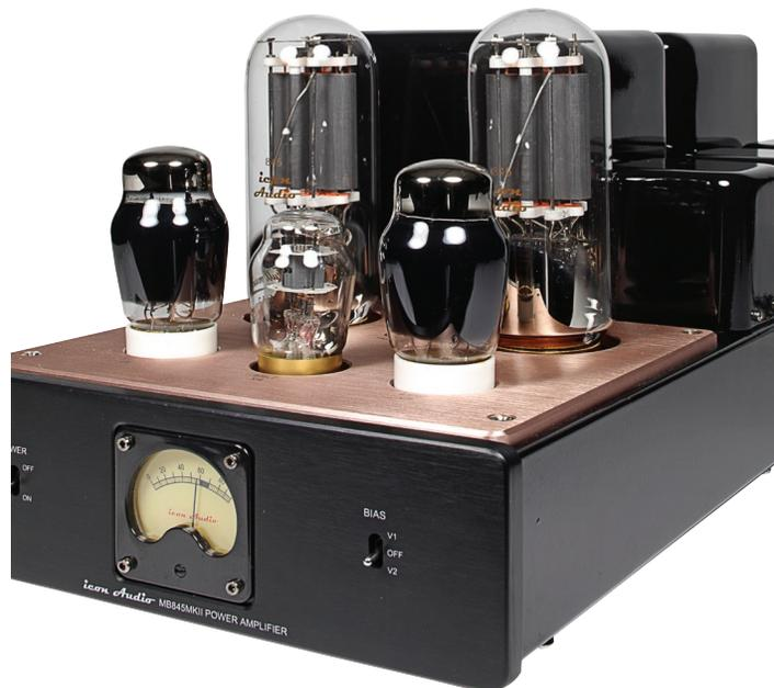
**Get the needle into the black and bias is correct, it's as simple as that. Tweaking bias on this 'fixed bias' amp is quick and easy.**
