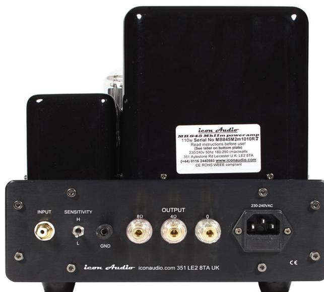
*At left is the Sensitivity switch, with H and L positions. Icon Audio recommend it is set in the down position to L, that gives most feedback and lowest output impedance (best Damping Factor).*
