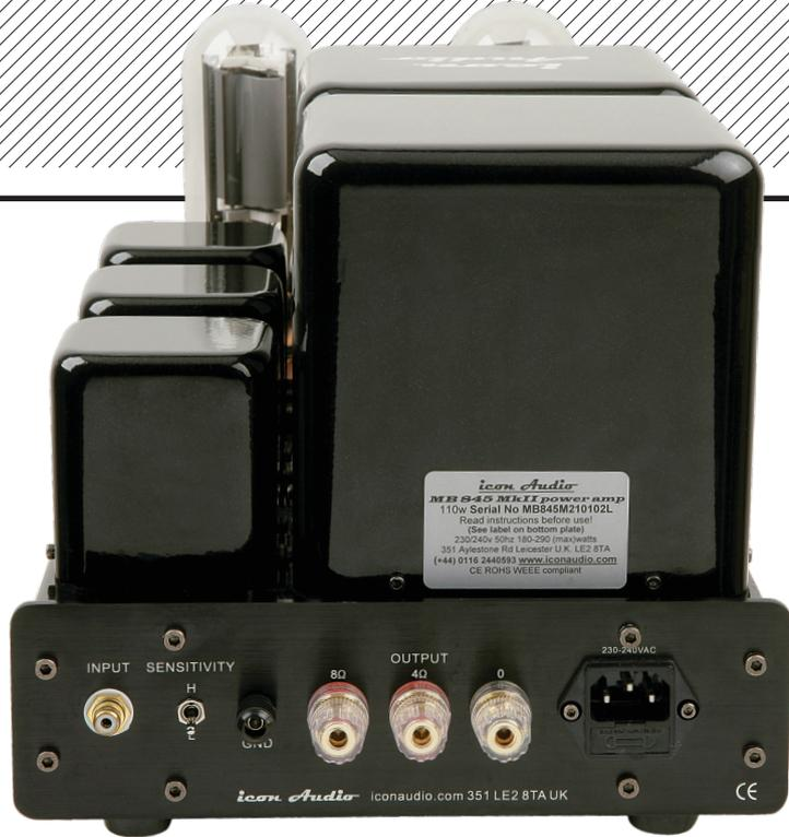
ABOVE: High/low sensitivity switch allows matching with passive and conventional preamps. Input is single-ended while speaker terminals provide 4 and 8ohm taps
