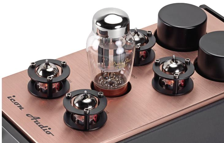
**Two low noise ECC88 (6922) twin-triodes per channel provide gain, and a big 6SN7 acts as a low impedance line driver. Input transformers at right step up the MC input. MM goes in direct.**
