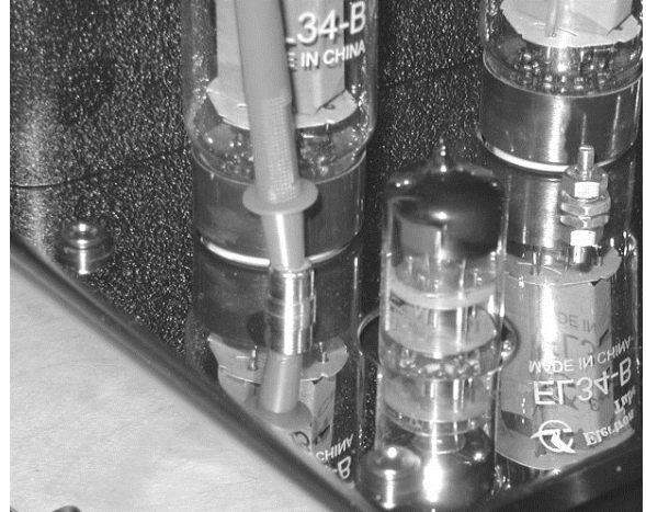
Showing a probe in output valve test point
