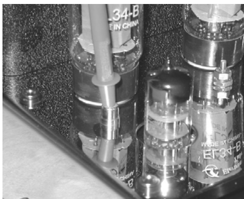
Showing a probe reading 1 st output valve
