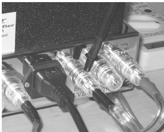
Making the 'earth' connection.
