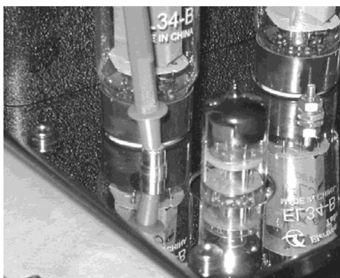
Showing a probe reading 1 st EL34
