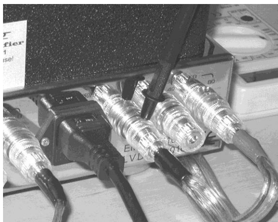
Making the 'earth' connection.
