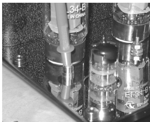
Showing a probe reading 1 st EL34
