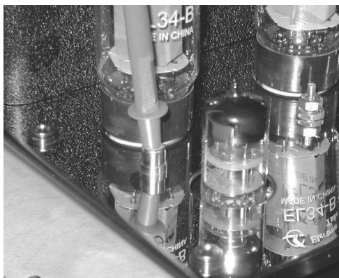
Showing a probe reading 1 st output valve
