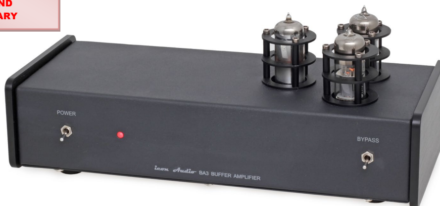
Showing the 0A2 on the left and the two 6N6 valves on the right.
