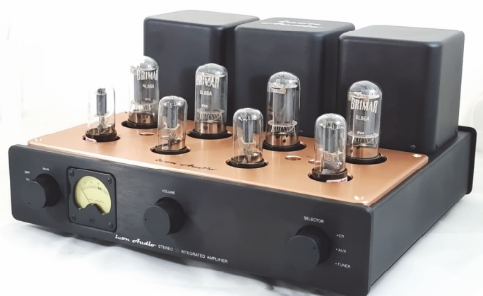
Shown with standard optional 6L6 and 6SN7 valves
