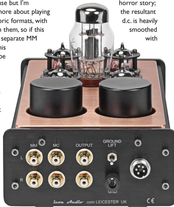
**Our rear shots shows gold plated, phono socket inputs and outputs, a ground lift switch to avoid hum, and a ground terminal. The circular canisters are screening cans around the input transformers.**
